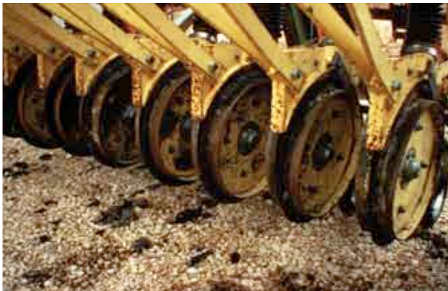
Depth control bands ensure that disc openers maintain a uniform planting depth when seeding native grass revegetation plantings.
